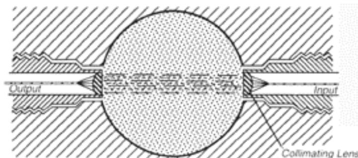
They support requirements where the path length will vary due to different media or for transfer of probes from one extruder to another. For purposes of economy, the two probes are identical and interchangeable.
