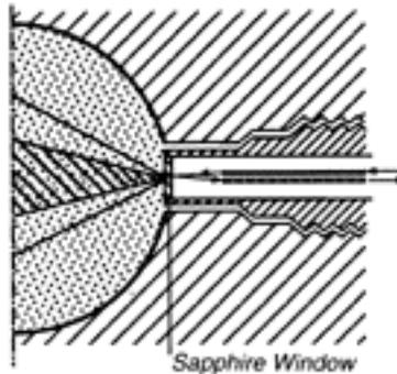
the RAMAN effect is maximized by an innovative concept on which a patent is pending. RAMAN spectroscopy is particularly useful on high-density media. Sensonetics' vastly improved collection efficiency allows RAMAN analysis of media that could not be analyzed previously.
